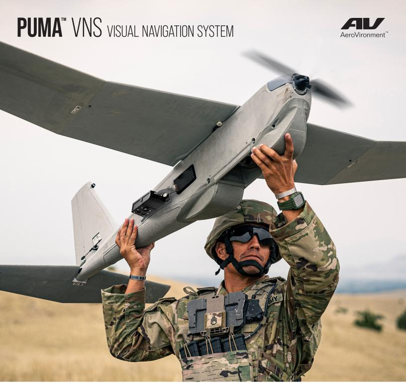
AeroVironment's Puma™ VNS is a visual-based navigation system for Puma 2 AE and Puma 3 AE small unmanned aircraft systems (SUAS). Puma VNS enables GPS-denied navigation across GPS-contested environments. The system performs Visual Inertial Odometry (VIO) through a suite of integrated sensors and an onboard compute module to determine the precise location of the aircraft during flight.
