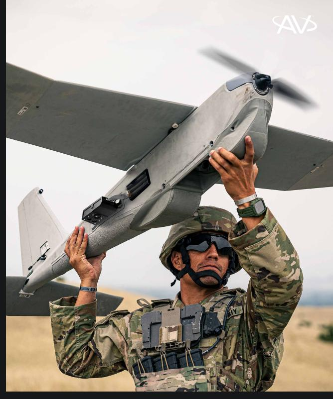
AV's Puma<sup>™</sup> VNS is a visual-based navigation system for Puma 2AE and Puma 3AE small unmanned aircraft systems (SUAS). Puma VNS enables GPS-denied navigation across GPS-contested environments. The system performs Visual Inertial Odometry (VIO) through a suite of integrated sensors and an onboard compute module to determine the precise location of the aircraft during flight.
