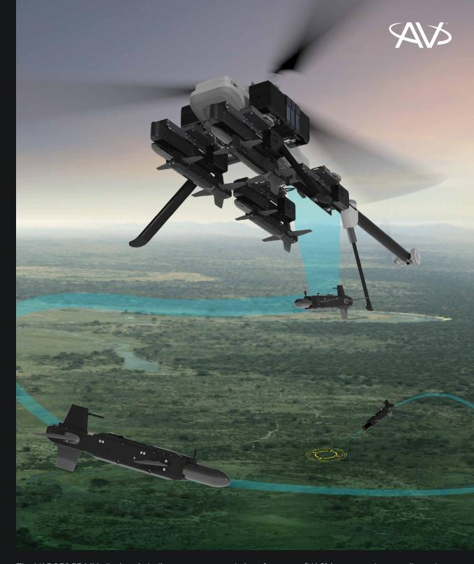
The VAPOR® 55 MX all-electric helicopter unmanned aircraft system (UAS) is extremely versatile and can be easily configured to support a variety of mission requirements. VAPOR's multi-mission, modular design offers class-leading payload capacity of 22 pounds with 60 minutes of endurance. Its unique rail mount enables quick and easy integration of multi-sensor payloads, or a drop mechanism optimized for the delivery of munitions, including Shryke.
